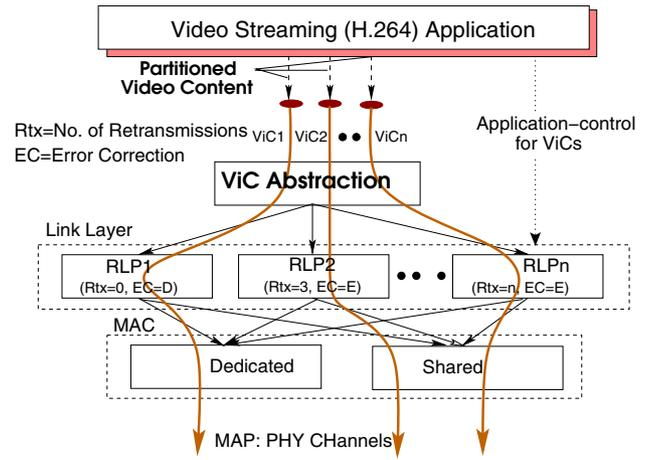
Fig. 3. Illustration of the Virtual Channels (ViCs) Abstraction in WWANs.
