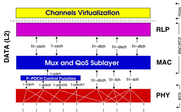
Fig. 4. Illustration of how Virtual Channels (ViCs) in MobiStream can operate on top of the logical link layer (dedicated or shared) channels and physical layer data channels in CDMA2000 3G WWANs. Video content is scheduled over ViCs in a proxy at or close to the PDSN node.
