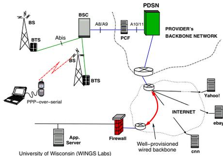
Fig. 10. Experimental Testbed Setup.
