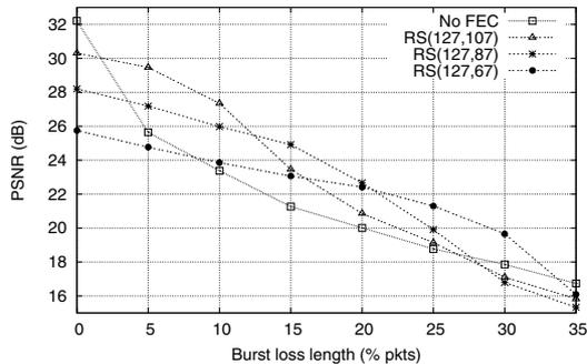
Fig. 12. Performance of dynamic application layer FECs using shortened Reed Solomon (RS) codes at different burst packet loss rates (% slice pkts) over an unreliable virtual channel. Vertical axis indicates the average luma PSNR (decoded) for *Foreman* video sequence.
