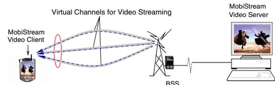
Fig. 1. Virtual Channels (ViCs) for Wireless Wide-area Networks.
